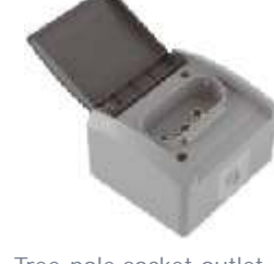
Tree-pole socket-outlet IEC 60884-1, CEE7 16A/440V; IP 44
