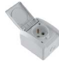
Two-pole socket-outlet "F" type (French standar) IEC 60884-1; CEE7 16A/250V; IP 44
