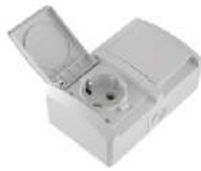
Double horizontal two-pole socket-outlet IEC 60884-1, CEE7 16A/250V; IP 44
