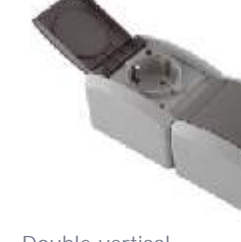
Double vertical two-pole socket-outlet IEC 60884-1, CEE7 16A/250V; IP 44
